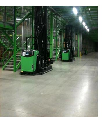
As robotic solutions are extremely precise, they demand a great deal from concrete floors – absolute flatness, no joints, and no movement are essential to ensure the necessary conditions for the full laser and camera/GPS operated automated forklifts to function with maximum efficiency (maneuverability, speed, etc.).
